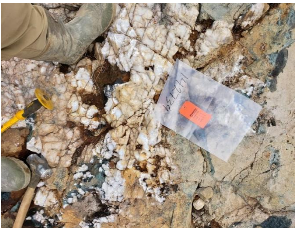
Flat-lying quartz lens with rusty patches of coarse-grained pyrite at Lot 25 trenches
