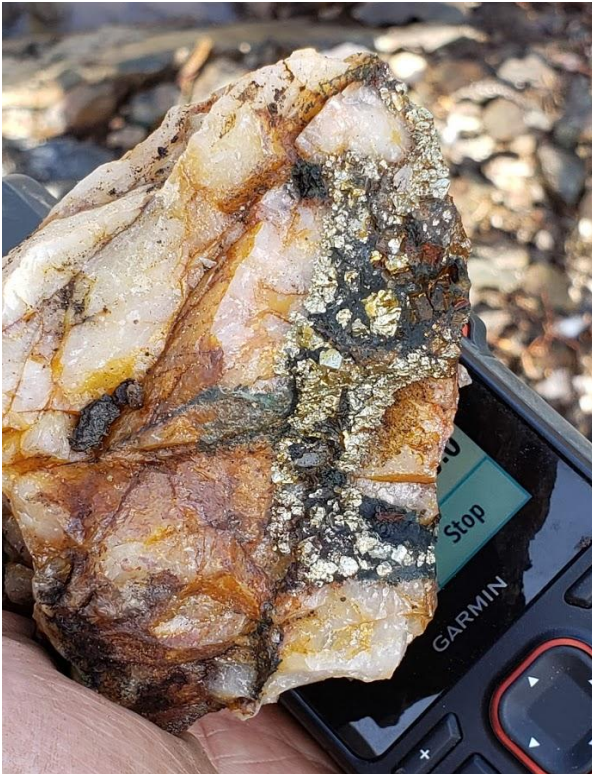
Quartz vein at Lot 25 Trenches with coarse-grained euhedral pyrite
