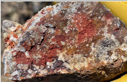
Close-up of barite and hematitic clay fracture filling
