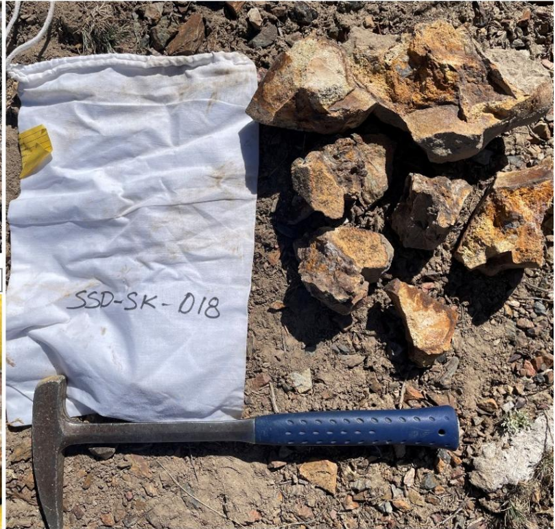
Limonitic, clay-altered lamprophyre with silica selvages Sample near the legacy 16.4 g Au/t sample
