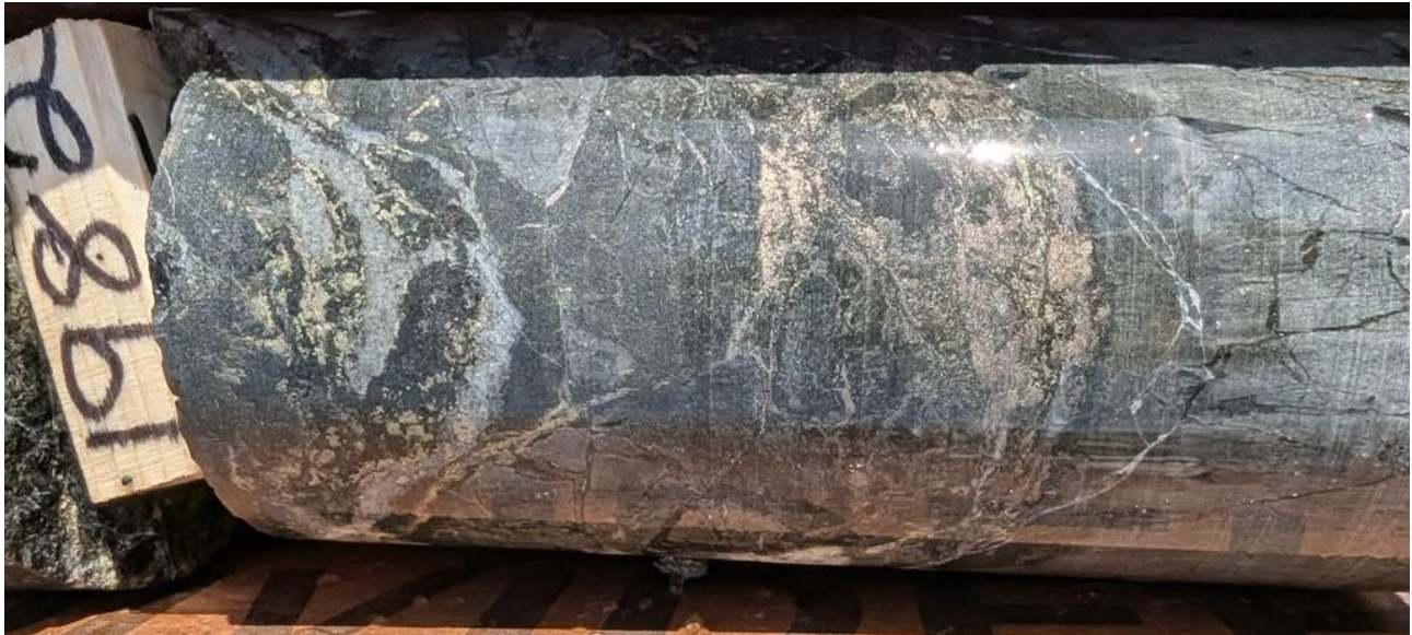
Figure 3: Visible chalcopyrite mineralization within the breccia zone in Hole MHB-37B at approximately 1,982 feet (604 metres).
